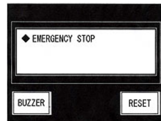
Example of an Interlock Screen. There are 25 kinds of interlock messages.
